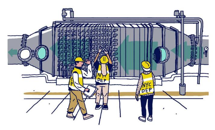
10. The city's water is treated with chlorine, but the chemical can create harmful byproducts when mixed with organic compounds. In the 1990s, ultraviolet radiation was identified as a safe and effective supplementary treatment. But for it to be evenly applied, the water must be moving at constant speed.
