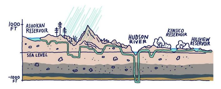
4. It can take 12 weeks to a year for water to wind its way to the city from the streams, tunnels, dams and reservoirs in the Catskills. All of it is delivered to the city by gravity alone.
